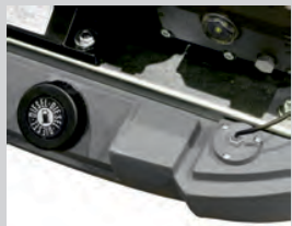
Controllo mancanza gasolio Low fuel warning device
