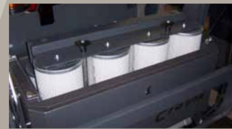
*GEMMA offers the opportunity to choose from two filter configurations. It is the action of the filter shaker that keeps cleaned the filter in both configurations.*
